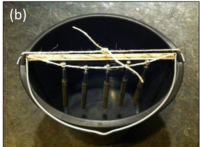
Fig. 5. (a) Steel bars immersed in tap water. (b) Arrangement for pre-rusting of steel bars in a bucket. (c) Steel bars placed in sealed bucket with water at the bottom for obtaining a superficial corrosion.
