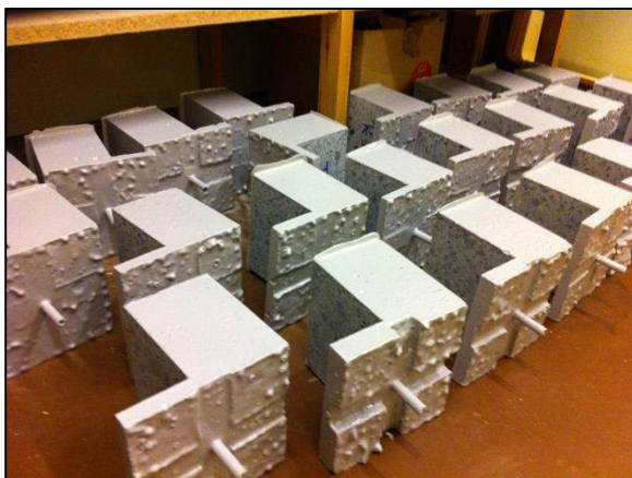
Fig. 14. The concrete specimens were placed in a climate chamber (25% RH and 20°C) in order to facilitate an accelerated ingress of chloride during exposure to NaCl solution. The dummy specimens were placed in the same chamber (not shown) and were oriented with the exposure surface (i.e. the surface without epoxy coating) facing upward. In contrast, the exposure surfaces of the specimens from series R and L were vertically oriented during the pre-conditioning as shown in the picture.
