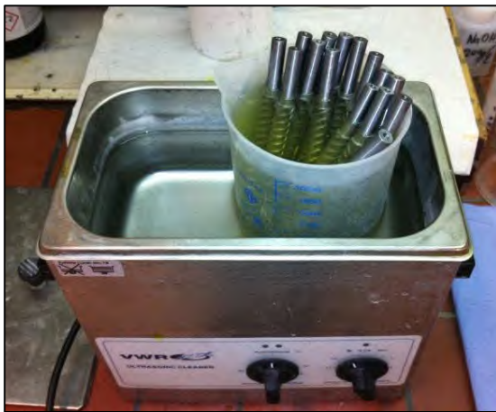
Fig. 3. Rebars were immersed in chemical cleaner solution ( \text{HCl} 1:1 + 3 \text{ g/l} urotropine) for 5 minutes and subsequently placed in an ultrasonic bath for 3 minutes.
