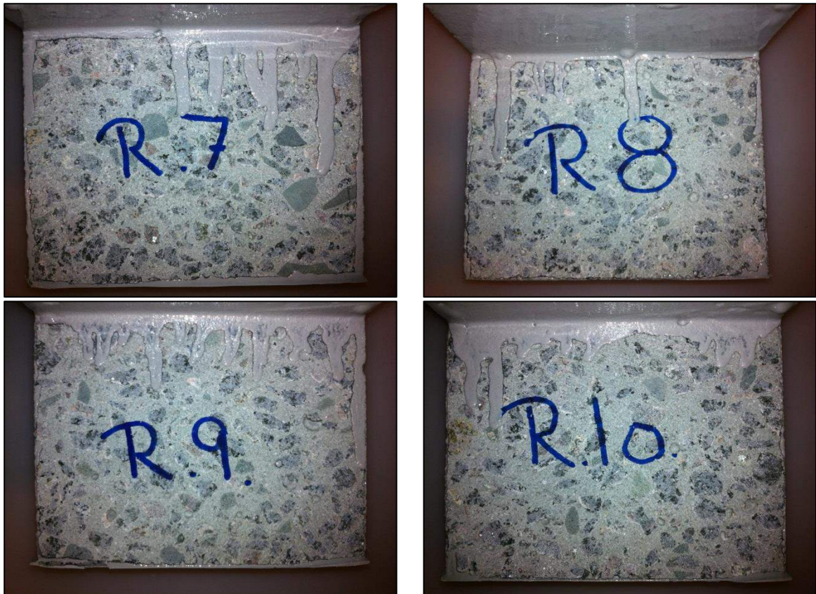
Fig. 16. Photographs of the surfaces of specimens R1 to R10 to be exposed to the 3.3% NaCl solution. The epoxy resin has run down on the cover surfaces of some of the specimens. The specimens were exposed to the NaCl solution in the conditions that are presented in the pictures.
