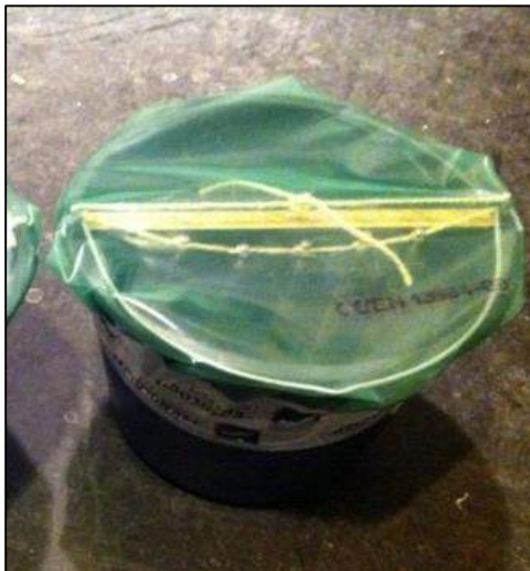
Fig. 5. (a) Steel bars immersed in tap water. (b) Arrangement for pre-rusting of steel bars in a bucket. (c) Steel bars placed in sealed bucket with water at the bottom for obtaining a superficial corrosion.
