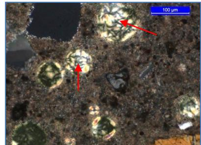
Figure 6: In other occasions thaumasite-like phases are present in the air voids.
