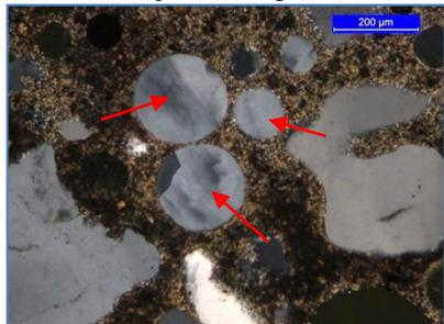
Figure 5: Occasionally air voids in the surface region are filled with gypsum. X-polarised light-
