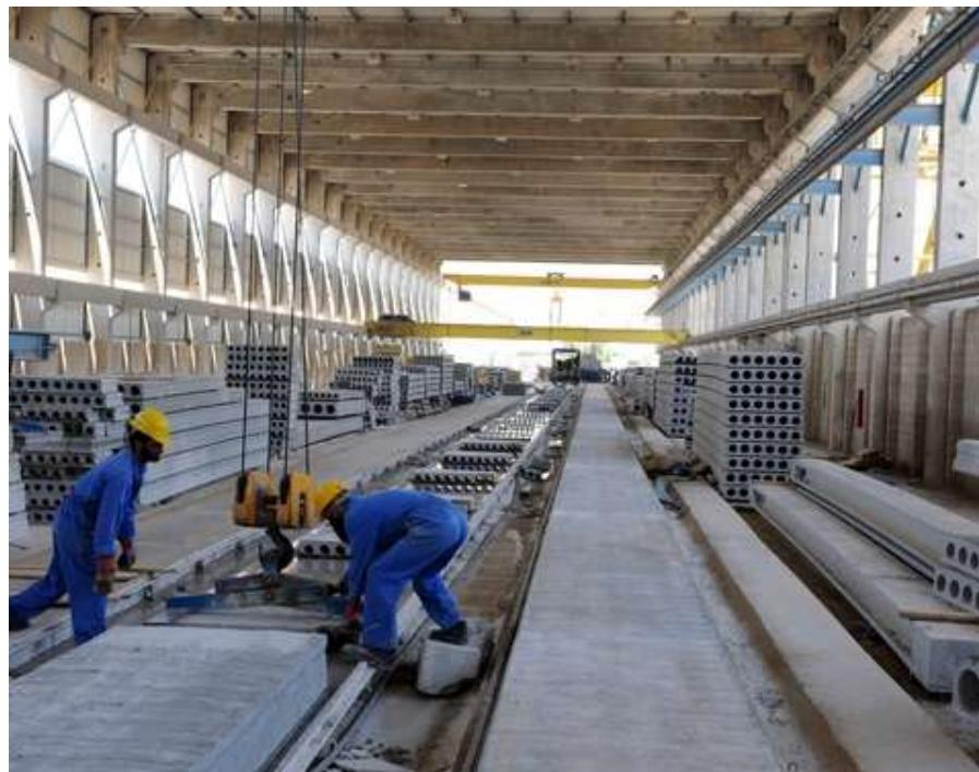
Production of pretensioned floor elements
