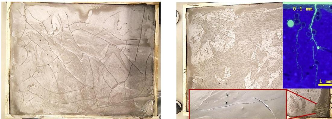
Figure 2 – Shrinkage cracks in UHPFRC. Fibre volume fraction: Left – 0%; Right – 4%.
