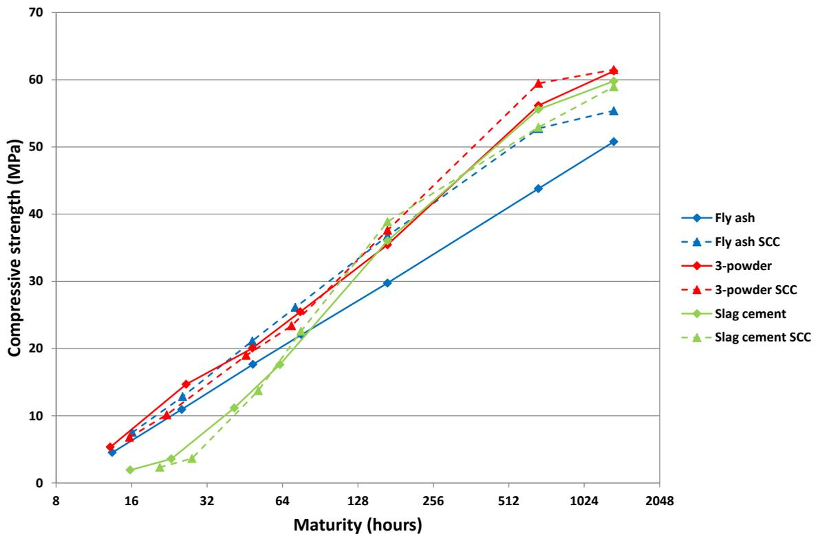
Figure 1 — Compressive strength development ( $\varnothing 150$  mm cylinders) of the six different concrete types tested.
