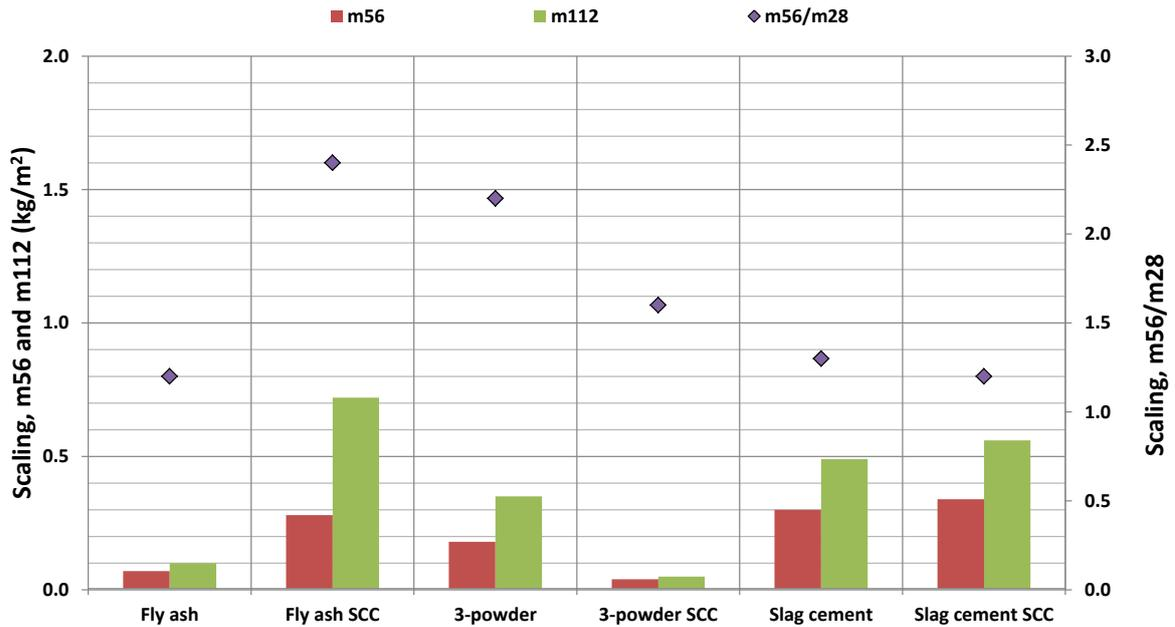
Figure 3 — Frost resistance of drilled cores taken from the small blocks.
